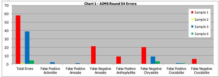
False Negative = Component has been missed. False Positive = Component has been incorrectly identified as present.
